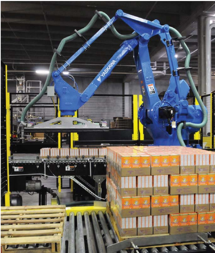
▲ VACUUM PLENUM. Shrink-wrapped corrugated trays of freshly cartoned mac and cheese are palletized by the robot’s end effector, whose two-zone vacuum plenum gives it considerable pick and place flexibility.
