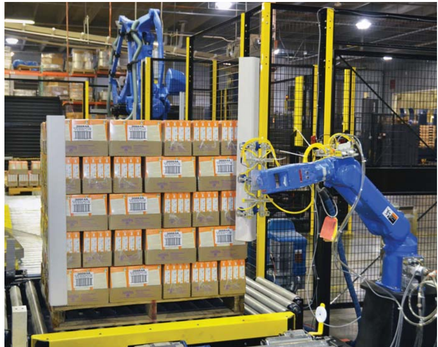
▲ ROBOTIC APPLICATION. Protective corrugated cornerboards are applied automatically by this robotic system just before stretch wrap is applied to the pallet.
