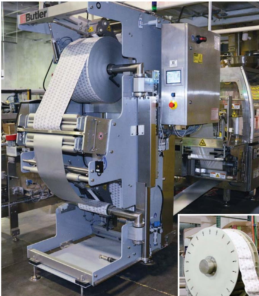
▲ AUTOMATIC SPLICING. Roll-fed film used to put powdered cheese into pouches is automatically spliced by the machine shown above. Exiting the pouching machine, cheese pouches are in bandolier format (at right).
