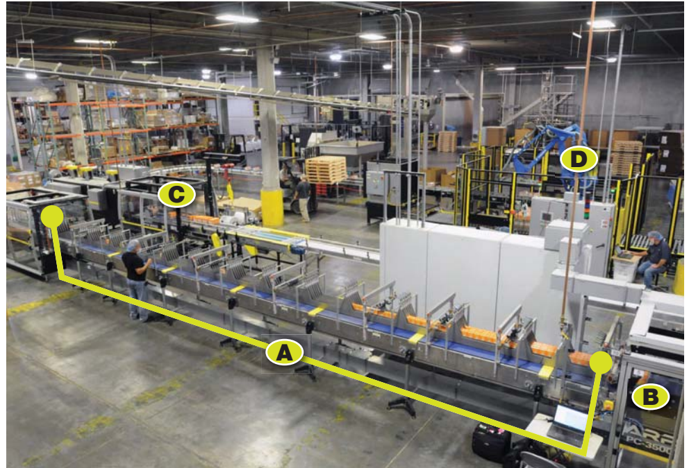
▲ BIRD'S EYE VIEW. The Bird's Eye view shows dynamic lane divide (A), PC-3500 case/tray packer (B), shrink wrapper (C), and robotic palletizer (D).
